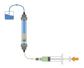
When sample loading is complete, connect the Superloop into the chromatography system flow path.
