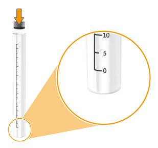
2 Fit the inner end pieces in the ends of the glass tube. Allow the inner end piece to push the movable seal into the glass tube.
