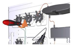
3 Remove the valve module.
