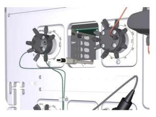
5 Connect the cable to the new valve module.
