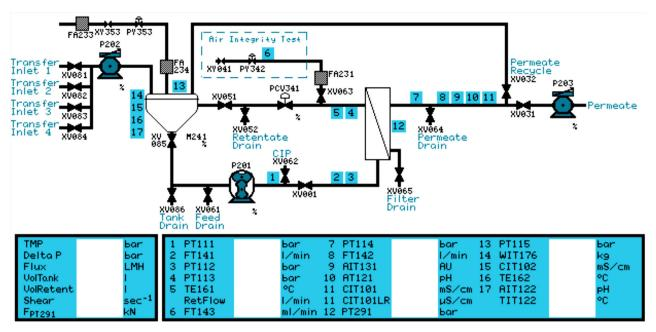
Fig 2. Example of a UniFlux flow scheme picture in the UNICORN software.
