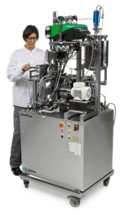
Fig 1. UniFlux 10 system configured for cassettes and with 10 L tank.
